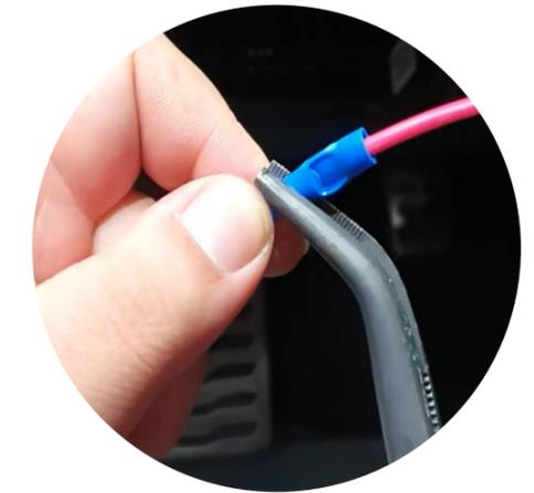
2. Pinch the terminal part with a tool such as a long nose.
