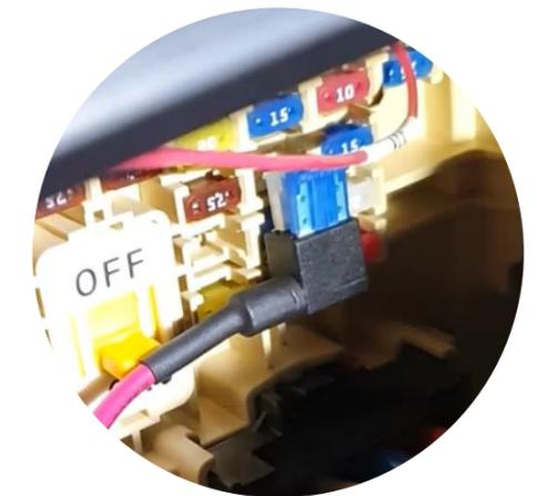
4. Finish by inserting the fuse holder into the removed seat.
