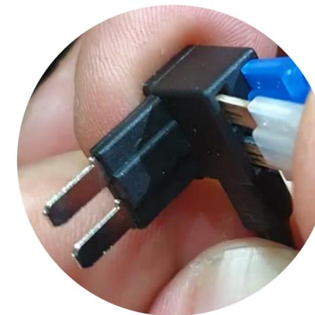
3. Remove the fuse from the original position and insert it into the empty space of the fuse holder.
